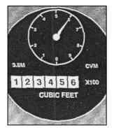
The direct reader meter, to the left, shows 6 digits with the least significant (right-hand) digit recording in hundreds of cu.ft. as the printed multiplier is X100, with a test dial showing 10 cu.ft per revolution.
